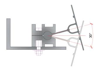
Our ball and socket design allows up to 30 degrees rotation to the front face of the rail.
