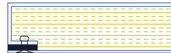
ULTIMA A1 - Outer tray with thermal break and mechanically fixed inner sheet
